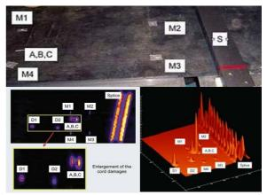
Fig. 8. Verification of visual damages of belt and splices illustrated in the Cord Guard system in 3D image [www.goodyearep.com]
