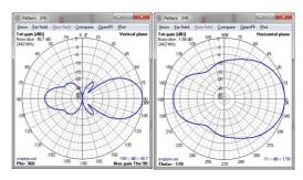
Fig. 8. Characteristics of radiating of the directional antenna: vertical (a), horizontal (b)
