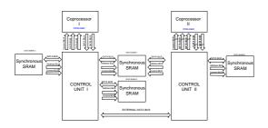
Fig. 2 FPGA processing module block diagram
