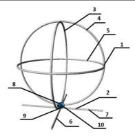
Fig. 1. Model of the omnidirectional loop antenna: 1
