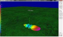
Fig. 10. Spatial characteristics of the directional antenna
