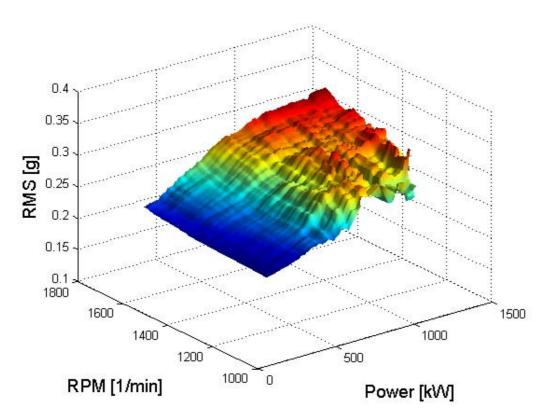
Fig. 5 RMS in relation to power and RPM presented for generator bearing in undamaged condition
