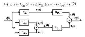
Fig. 3. Diagram showing generation of the linear and non-linear parts of the process.
