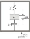
Fig. 2. A dynamic system with one degree of freedom subjected to a kinematic input [8]
