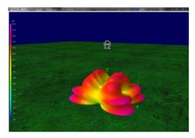
Fig. 5. Spatial characteristics of the omnidirectional antenna
