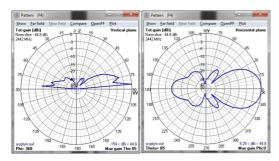
Fig. 9. Characteristics of radiating of the directional antenna above the surface: vertical (a), horizontal (b)
