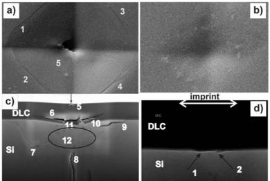
Fig. 3. SEM images of two impressions: a) top view 100b, b) top view 100d, c), d) correspondig cross-section made by FIB system, numbers indicated surface and cross-section failures
