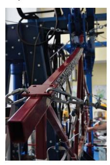
Fig. 12. deformed truss after first loading cycle
