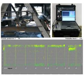
Fig. 2. The Belt Guard system, and the image after belt scanning (belt conveyor ST2200, 2307m x 1500mm) [www.beltscan.com.]
