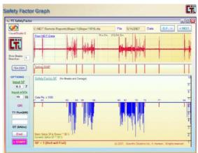
Fig. 5. Damages diagram of the tested belt (red) and the safety factor (blue)
