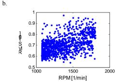
Fig. 4 RMS in relation to rotational speed (RPM) for bearing: a. undamaged, b. damaged
