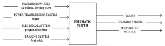
Figure 1. Interactions in the pneumatic system.
