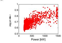
Fig. 3 RMS in relation to power for bearing: a. undamaged, b. damaged relation to the power is greater than for RPM
